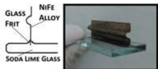
Figure 3: Sample & schematic of TVP glass-metal sealing
