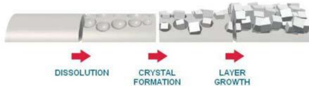
Figure 9: Illustration of the Partial Support Transformation process
